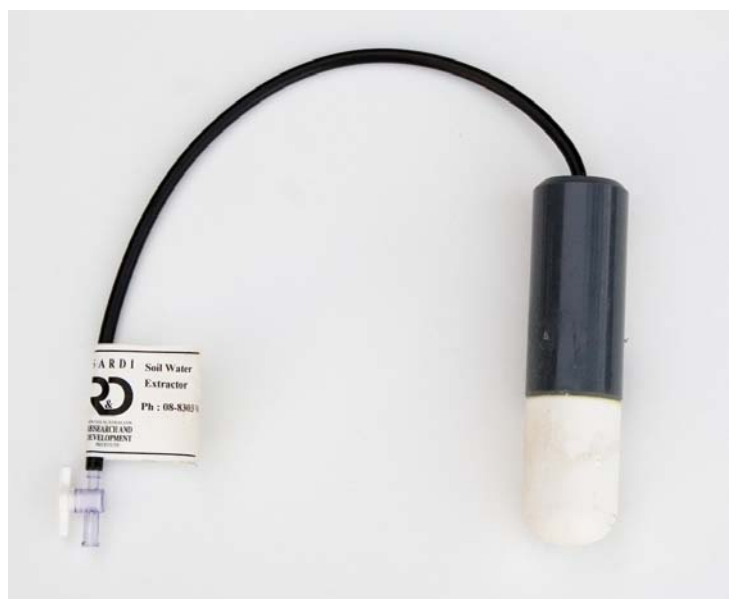
Figure 6 : SARDI/Sentec 40mm SSET ( SoluSAMPLER™ - www.sentek.com.au ).
