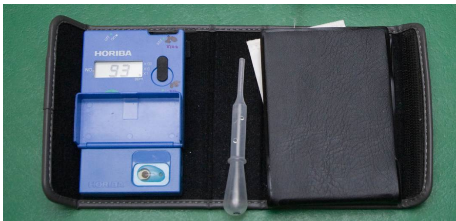
Figure 26 : Horiba Cardy nitrate meter reading a sample
