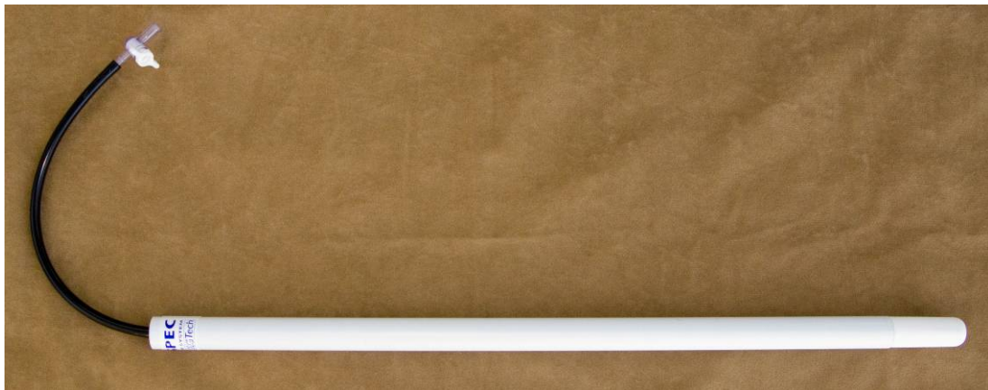
Figure 12 : Soil Spec 20mm SSET manufactured by J.K.G Tech.
