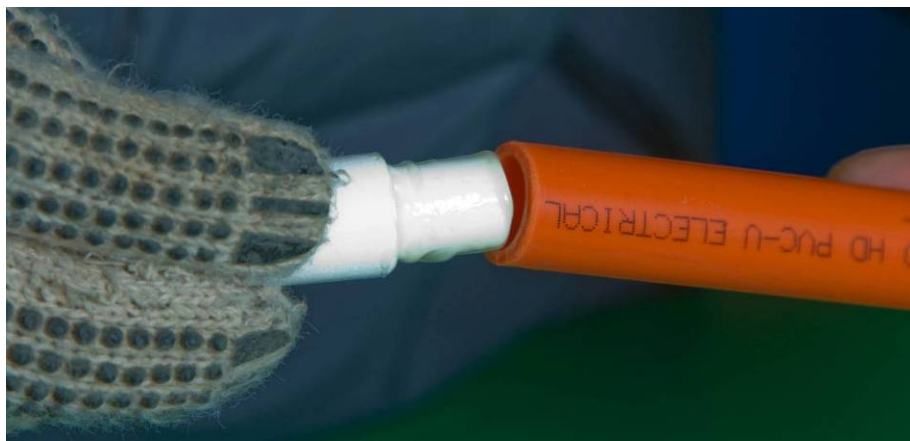
Figure 24 : Making a ceramic sampler; gluing a ceramic tip into electrical conduit
