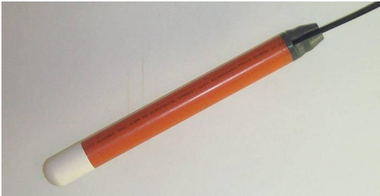
Figure 5: CSIRO 40mm SSET constructed since 1995 (Poss, 1995 & Deery et al, 2004). The sampler has an installation cap (grey) attached to the tube.
