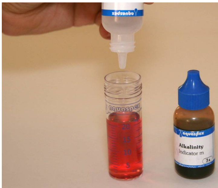
Figure 28 : Measuring the total alkalinity using an Aquaspex test kit. Similar colour change test kits are also available for calcium and phosphorus.
