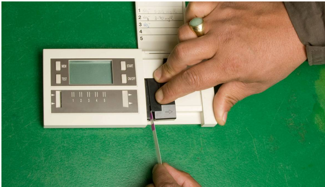
Figure 27 : Inserting a test strip into the Merck RQ Flex meter to take a nitrate reading
