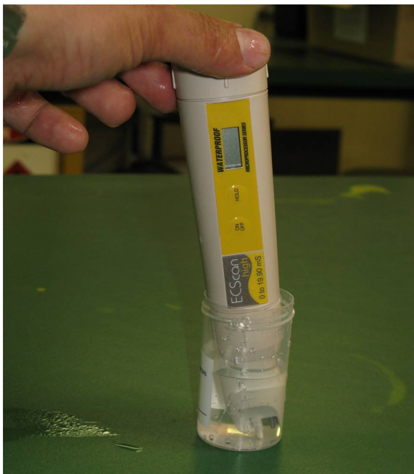
Figure 21 : Measurement of the salinity of soil solution with a EC meter
