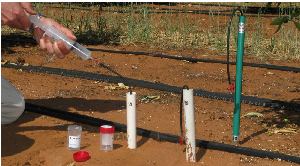
Figure 23 : Extracting soil solution from a set of 20mm wide soil solution extraction tubes.
