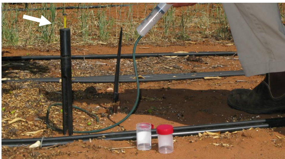
Figure 22 : Extracting soil solution from a FullStop wetting front detector. The raised yellow spike (white arrow) has signalled that the wetting front has reached 30cm depth.
